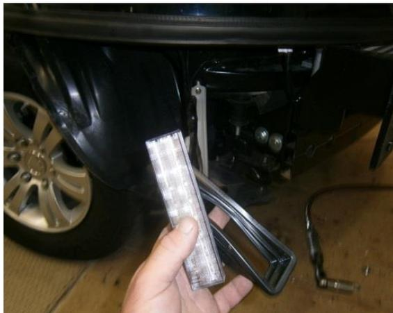
Attach wiring harness supplied to park and indicator wiring behind headlight using yellow wire for indicator, brown for park and white for earth. Attach using solder or wiretap connectors supplied. Attach indicator to terminals. Yellow to yellow, white to white and black to brown.
