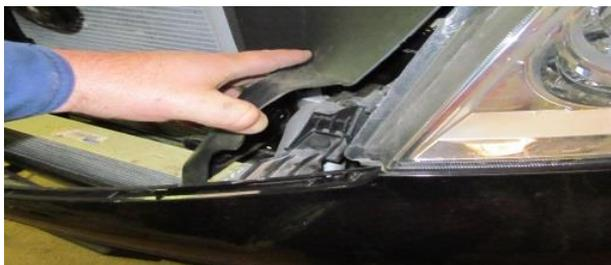
Remove all clips and screws from topside, wheel arches and underside of bumper. And remove bumper.
