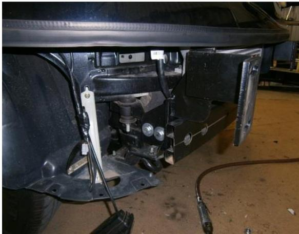
Loosen crashbox and slide bulbar brackets behind and beside chaise use 12mm\*130mm bolts with 12mm flat washers and 12mm nylock nuts . tighten all bolts
