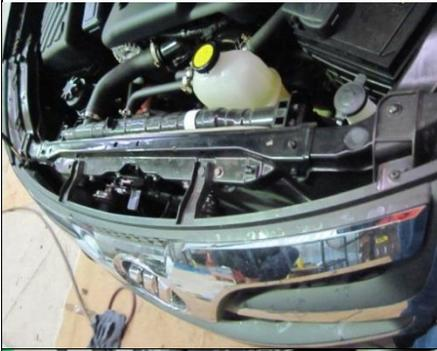
Remove plastic radiator cover to expose clips and screws in top of grill
